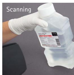
**SCANNING:** Hold the bottle and scan at a 45°–90° angle, 2"–6" from the bottle.
