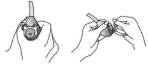
**Replace:** Position the bottom of the new plate to the socket of the chestpiece. Snap the top firmly into place.
