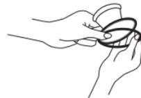
**Threaded (Metal) Rim:** Turn rim counterclockwise to remove. Replace with new diaphragm and reattach rim by turning clockwise until tight to re-assemble.
