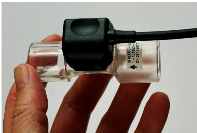
FIGURE 12-F: FLOW SENSOR CONNECTION TO FLOW SENSOR CABLE
